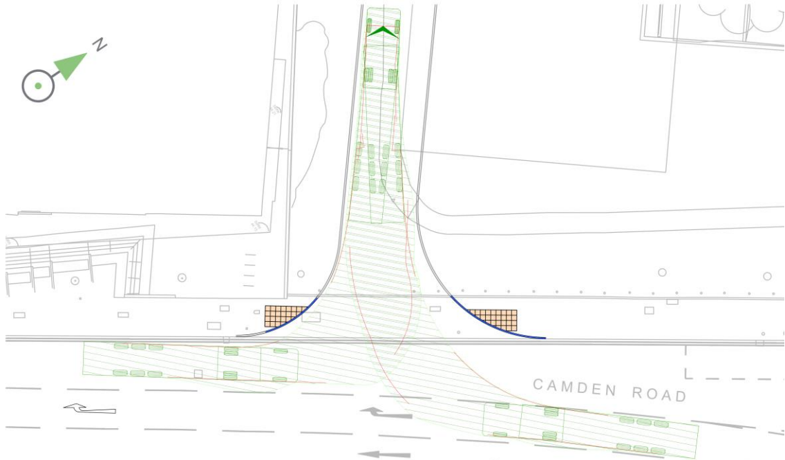
Figure 12 - ACCESS LEFT & RIGHT TURN 16.5m ARTICULATED VEHICLE
