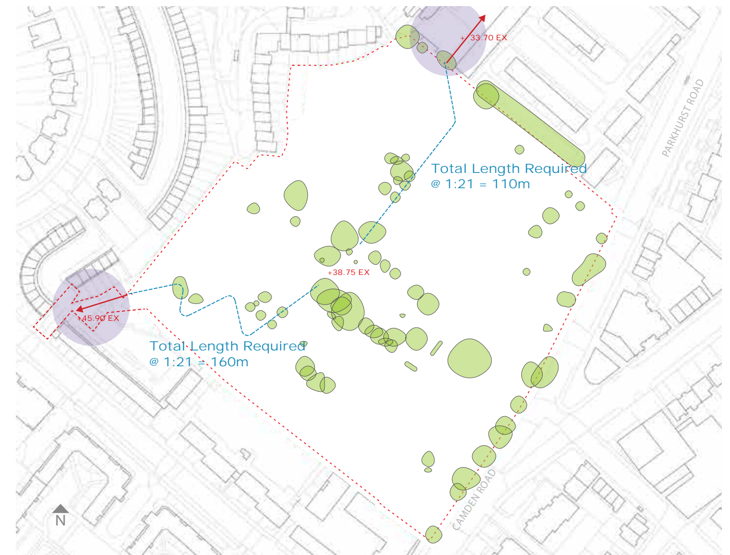
Plan showing the length required to create an accessible gradient between existing levels of the existing trees to be retained.
