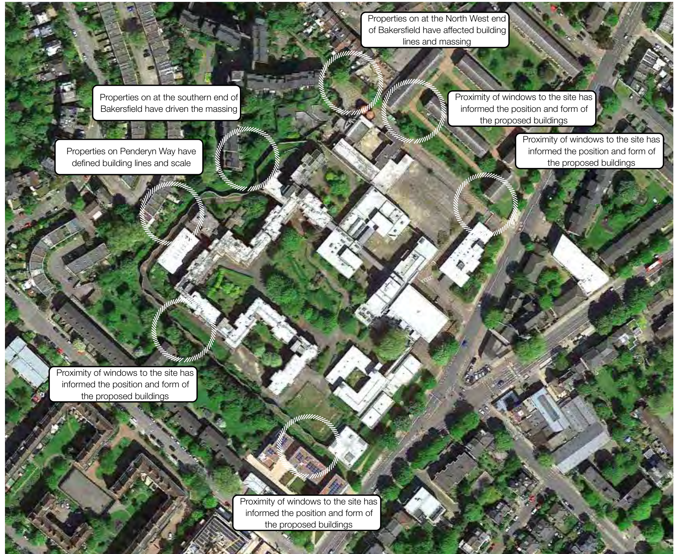
Aerial photograph showing existing relationship with nearest neighbours
