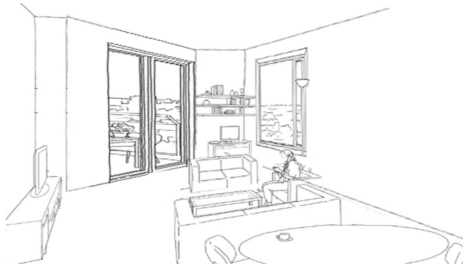
Our approach to creating dual aspect units by creating a projecting corner with the same geometry as a standard corner
