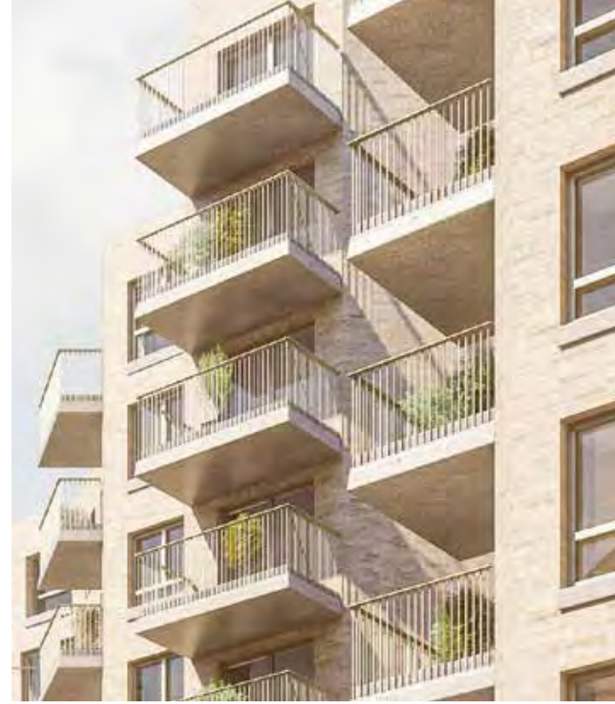
● Concrete balconies with metal guarding and handrail
